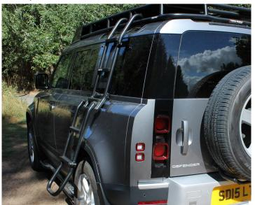
Made of a folding construction with dual securing methods and a key locking mechanism. Requires drilling of the trim panels below the rear window to allow installation into the existing body mounts beneath. When deployed, the height from the floor to the lowest step of the ladder is 585mm at normal ride height (660mm at max and 550mm at min).
