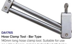
on rubber hoses, making it ideal for both brake and fuel lines together with coolant hoses. Steel construction with round chrome plated bars to help prevent damage.
